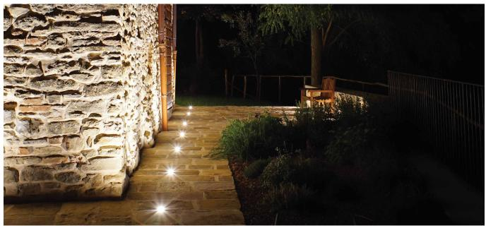
Flush-fitted in polished 304 steel with powerful LEDs suitable for decorative lighting and as step markers. Anti-glare radial diffuser, can be installed indoors and outdoors. Mounting with formwork for brickwork.
